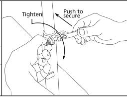
Fasten legs in place by tightening tension screws on the locking clamps at the base of each leg and push clamp lever down to secure.
