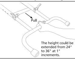
Grasp leg base and pull to extend leg to desired height. Make sure locking pin is secured in on the length adjustment holes.
