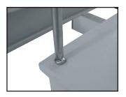
16) Place the cover back onto the electrical control box. Using a Phillips head screwdriver, replace the screws and tighten to secure in place.
