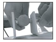
Remove the locking pin, slide to the top of the electric lift shaft into place between the mounting brackets, and reinsert the locking pin through the mounting brackets and the top of the electric lift shaft.
