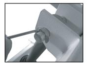
Use a flathead screwdriver (or other pointed tool) to pull out the snap rings from the locking pins on the electric lift mechanism.
