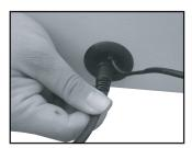
Slide the cord from the new electric lift mechanism through the rubber gasket on the electrical control box.
