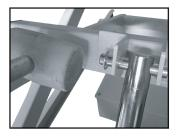
11) Using a hammer, tap both locking pins into place.
