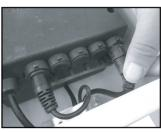
Unplug the cord that connects the electrical control box to the electric lift mechanism.
