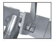
12) Using a flathead screwdriver (or other pointed tool), replace the snap rings to secure the locking pins.
