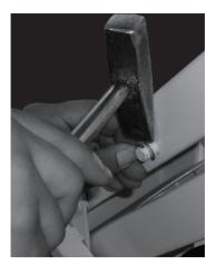
13. Tap in retaining clips onto the clevis pin at the right position.
