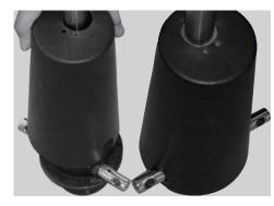
8. Cover the inner core of the hydraulic pump by using the plastic outer casing.
