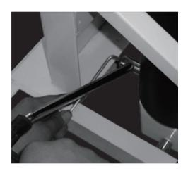
14. Attach the foot lever to the new hydraulic pump.
