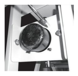
11. Use a wrench to replace the bolts on the bottom of the hydraulic pump.
