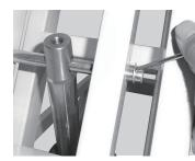
Use a sharp tool to pull out the retaining clips from the clevis pin on the hydraulic pump.
