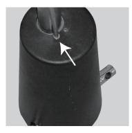
Using the screw from step 6, attach the plastic outer casing to the inner core.
