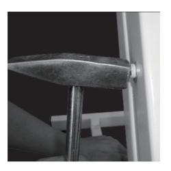
12. Using a hammer tap in the clevis pin.
