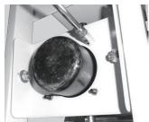
Use a wrench to loosen the bolts on the bottom of the hydraulic pump.
