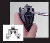
**HOW:** Turn off clipper and snap off the detachable blade.
