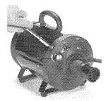
5. With the screw holes on the front panel and main body of the dryer aligned, replace the front panel. Insert screws into screw holes and use a Phillips-head screwdriver to tighten all four, securing the front panel in place.
