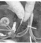
4. Install the new fuse and screw the two pieces of the fuse housing together to close.
