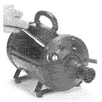
Using a Phillips-head screwdriver, loosen the screws on the front panel of the dryer. Gently remove the front panel from the main body of the dryer.
