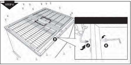
4. Secure the Front Panel (D) to the assembled panels using bolts J and K. The smaller (J) bolts should connect from the front, the Larger (K) bolts from the back. Use the two Allen Wrenches (E) secure the bolts as shown.
