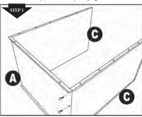
Connect the Side Panels (A) to the Top and Bottom Panels (C) using Screws (L). Note: the panel sides with the metal edging should all be facing out. The flat sides should face in.
