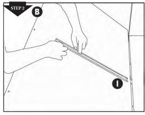
2. Connect the Dividing Panel Holder (I) to the Back Panel (B) using Screws (L). Note: The end where the Dividing Panel Holder (I) is closer to the edge of the Back Panel is the bottom end. To ensure safety use the Screw Caps (M) to cover the screws on the back side of the Back Panel.
