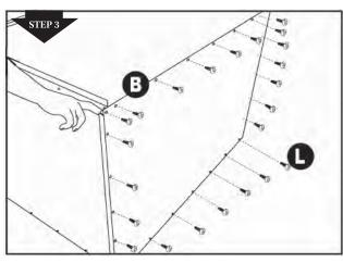
3. Connect the Back Panel (B) to the assembled panels using Screws (L).
